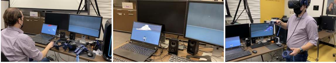
Fig. 1. Single-user CR prototype for reservoir engineering data visualization. The user performing analytical work on a laptop transit 3D reservoir model from standard monitor to VR space to increase working space and improve spatial perception.
